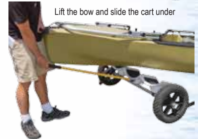
Leave the handle in place while moving the boat
